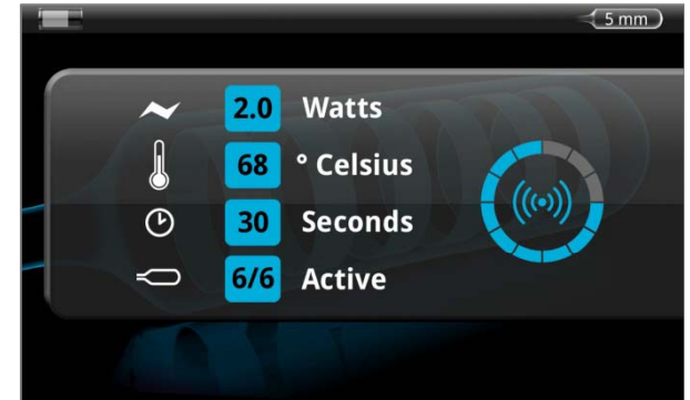
Active Treatment screen, indicates power, temp, time and # of electrodes active
