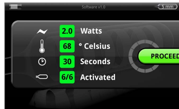
End of Treatment screen, data captured and saved to memory includes power, temp, time and # of electrodes activated
